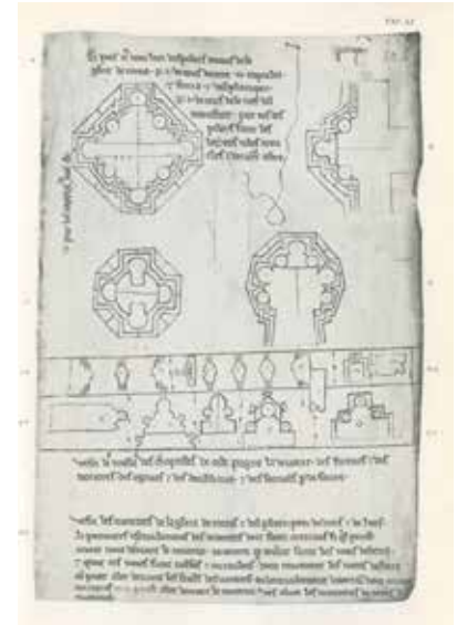
Fig. 1 Villard de Honnecourt, Plate 63 from the Album de Dessins et Croquis, ca. 1235. Tower pillars of the church of Reims as well as profiles of the chapels, window arches and cross ribs. The many drawings, which are accompanied by explanatory comments, document the architecture and construction of the time. They were created during Honnecourt's travels through Europe and form a kind of textbook on medieval construction.
