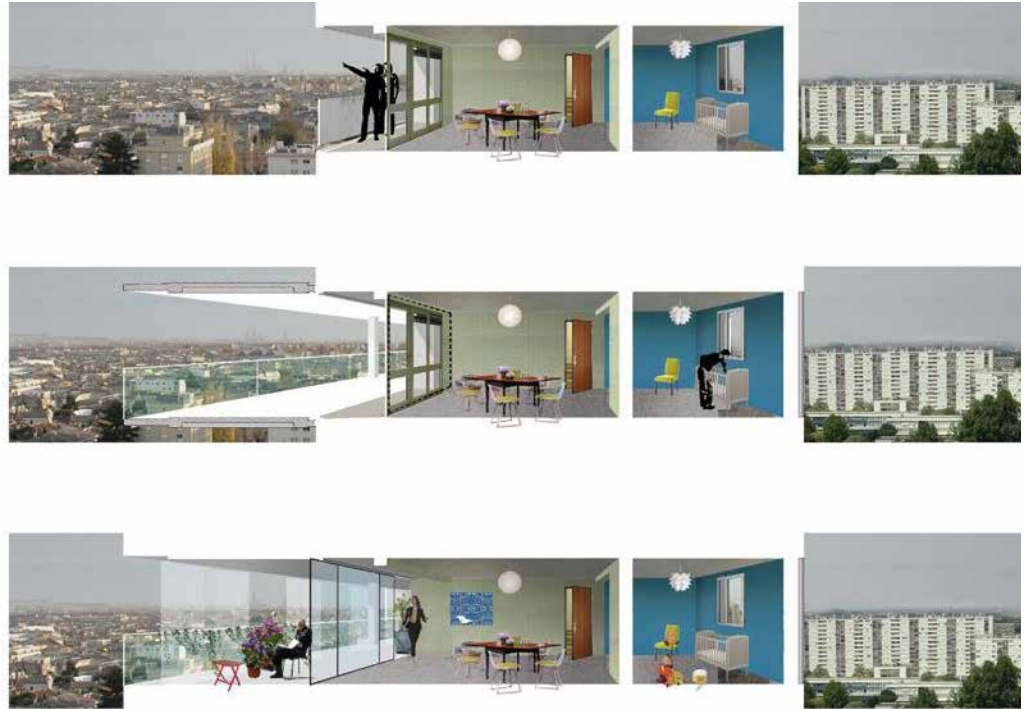
Fig. 5 - From above: existent and transformation projects. Perspective section of the project 'from the inside'. Transformation of 530 dwellings, buildings G, H, I, quartier du Grand Parc, Bordeaux, France, 2017. Source: www.lacatonvassal.com .
